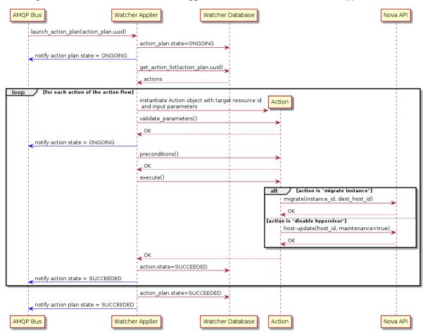
The *Watcher Applier* will get the description of the flow of *Actions* from the *Watcher Database* and for each *Action* it will instantiate a corresponding *Action* handler python class.
