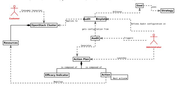
Here below is a diagram representing the main objects in Watcher from a database perspective:
