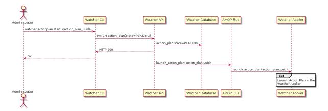
A message is sent on the AMQP bus which triggers the Action Plan in the Watcher Applier:
