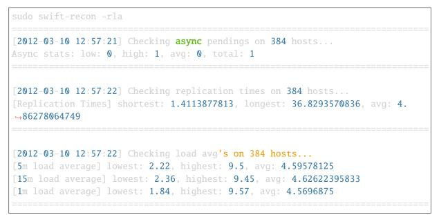
In the example above we ask for information on replication times (-r), load averages (-l) and async pendings (-a). This is a healthy Swift system. Rules-of-thumb for good recon output are:
