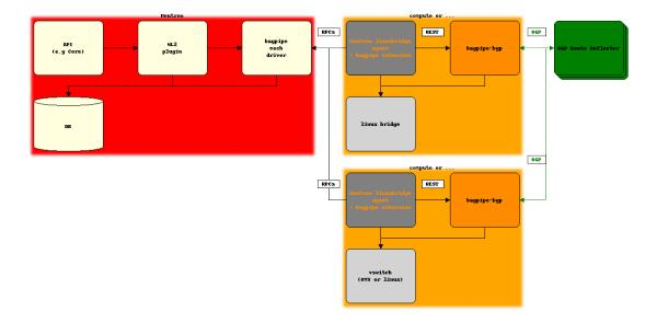
This solution is currently supported with the linux networking stack (i.e. with the linuxbridge agent enabled with bagpipe extension, and *BaGPipe-BGP* driver for the linux bridge VXLAN implementation). The approach would be easily extended to support OpenVS witch as well.
