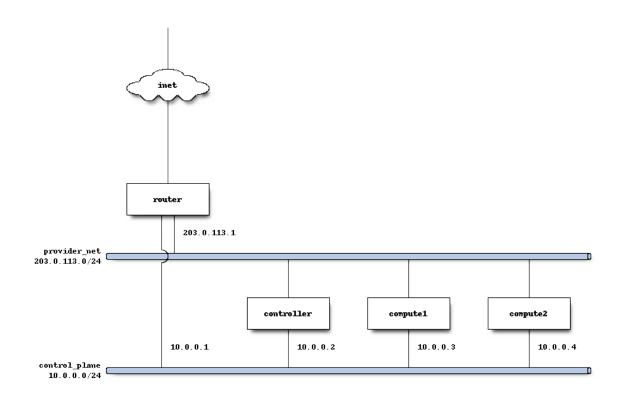
On a compute node, the first interface, eth0 is used for the OpenStack management (API, message bus, etc) as well as for ssh for an administrator to access the machine.
