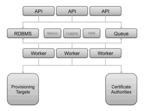
The API node(s) handle incoming REST requests to Barbican. These nodes can interact with the database directly if the request can be completed synchronously (such as for GET requests), otherwise the queue
